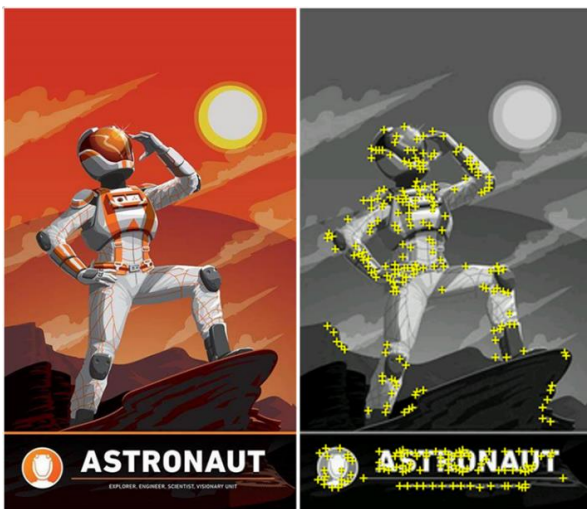
Fig. 1. The target image for AR projection. Left: Original version. Right: Feature points shown represented with dotted point.
