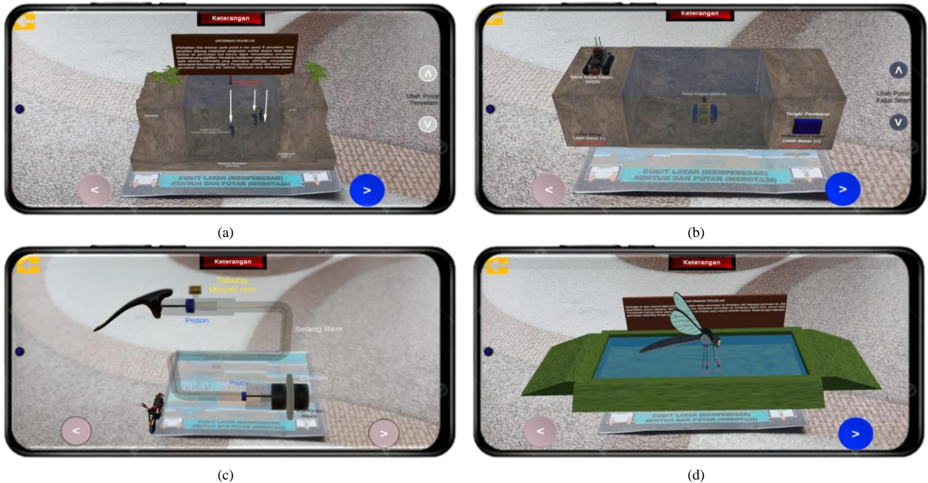
Fig. 2. AR of static fluid: (a) hydrostatic pressure; (b) the Archimedes principle; (c) Pascal's principle; (d) surface tension.
